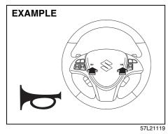
Press the horn pad on the steering wheel to sound the horn. The horn will sound with the engine switch in any ignition mode.
